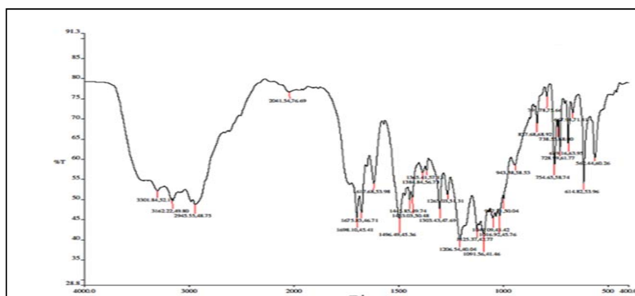
Fig 7: FTIR spectra of Amlodipine Besylate ODFs prepared using HPMC E3
