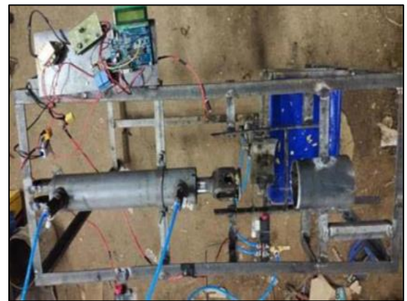
Fig 13: Pneumatic Pineapple peeling (Madhankumar et al. , 2021)
