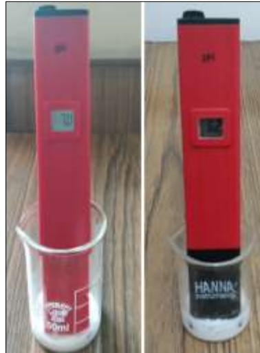
Fig 1 & 2: Milk samples showing milk pH with digital pH meter
