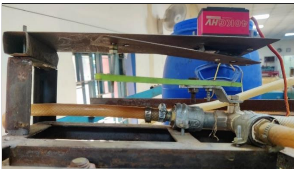
Fig 7: Variable rate servo motor operated spraying system
