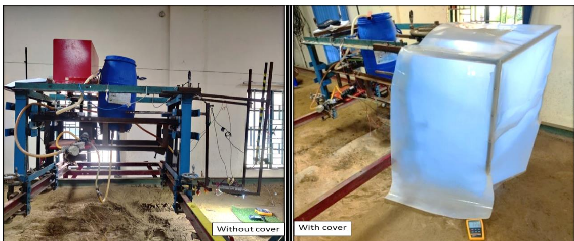
Fig 16: Developed prototype of sensor- based weed detection and herbicide applicator system
