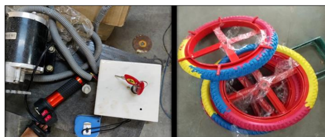
Fig 4: Motor and pneumatic wheels for sensor- based herbicide applicator
