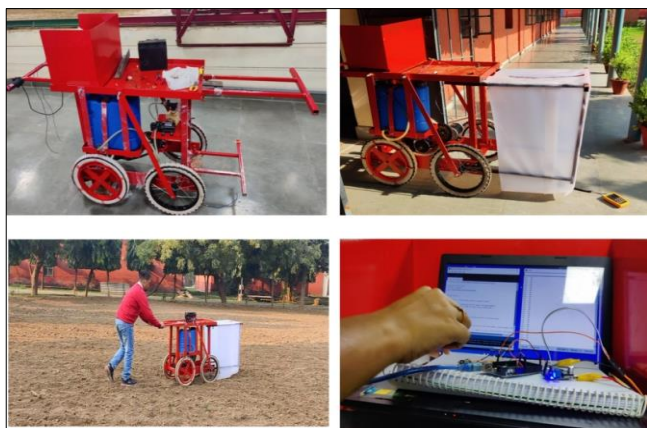
Fig 18: Developed prototype of sensor- based weed detection and herbicide applicator system
