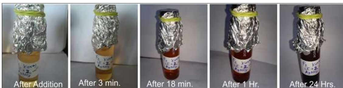
Fig 1: Change in colour of silver nitrate solution after addition of kusalgrass extract
