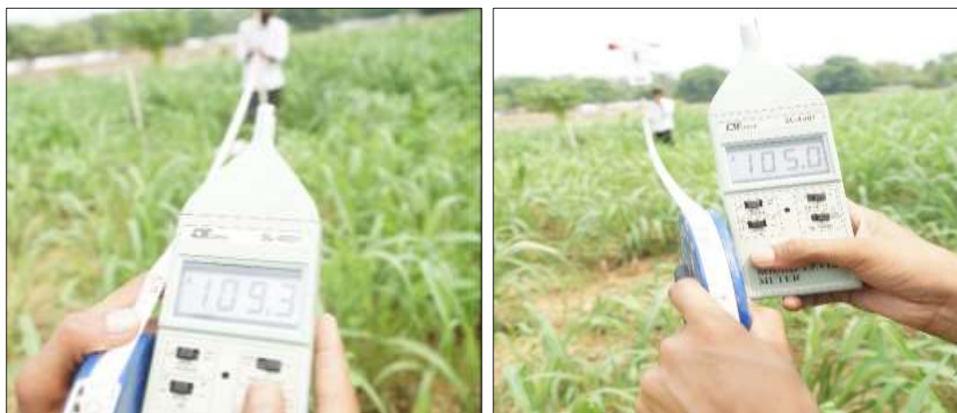
Fig 17: Testing sound pressure level at different distance
