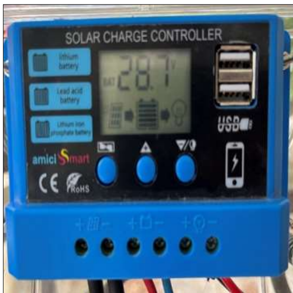
Fig 2: Solar charge controllers
