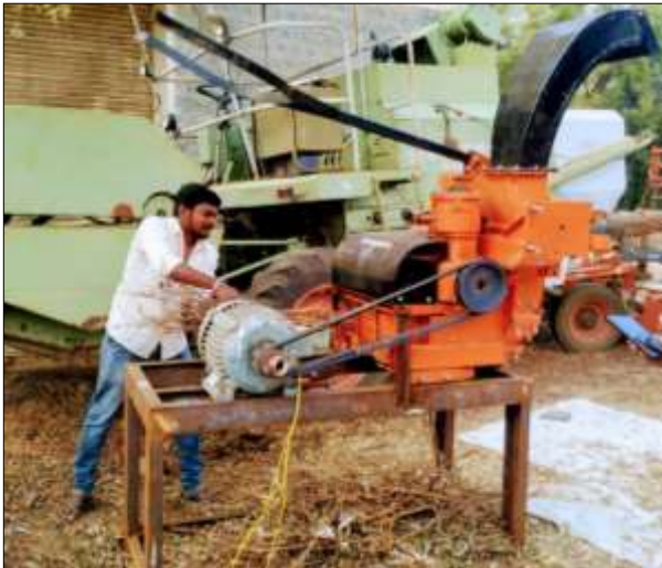
Plate 1: Laboratory evaluation of cotton stalk shredder
