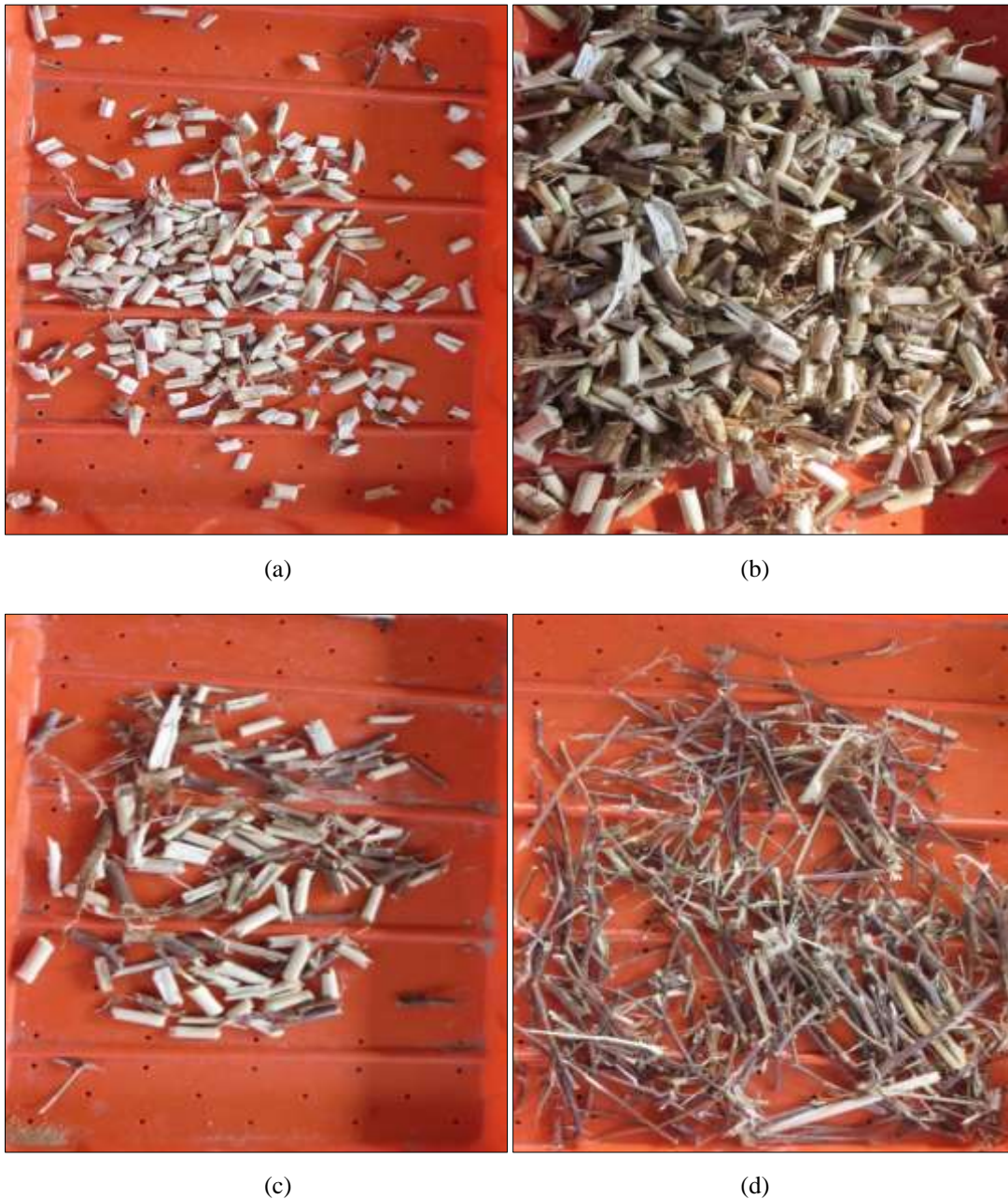
Plate 2: Different lengths of shredded cotton stalk (a) <10 mm (b) 11-25 mm (c) 26-35 mm (d) 36-150 mm
