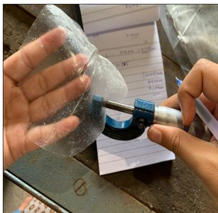
Fig 1: Measurement of thickness using micrometre
