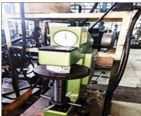
Fig 8: Apparatus for Hardness test
