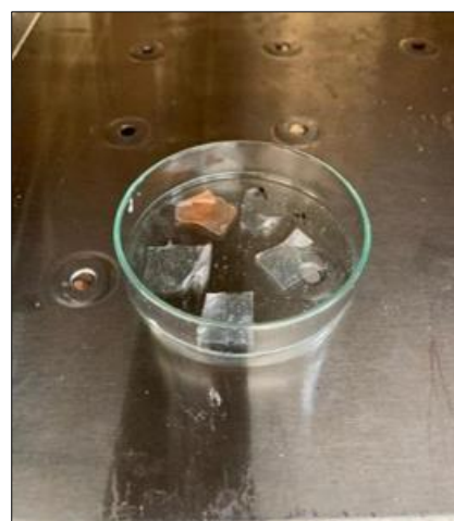
Fig 2: Moisture content measurement
