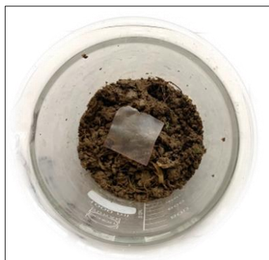
Fig 5: Soil Burial Test
