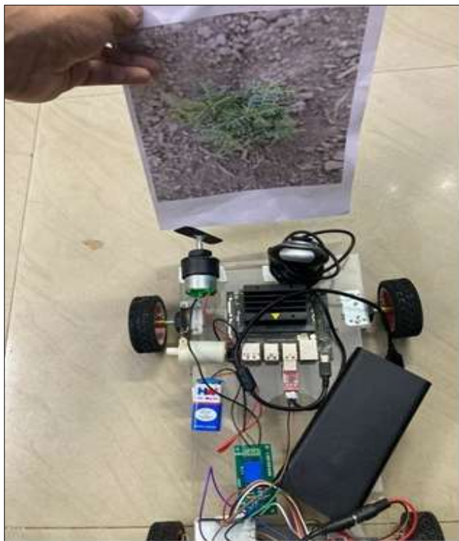
Fig 20: Robot detecting weed and stops
