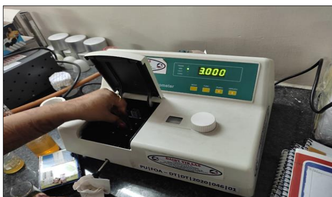
Fig 10: UV- visible spectrophotometer (single beam) in Department of Dairy & Food Technology, Parul Institute of technology, Parul University
