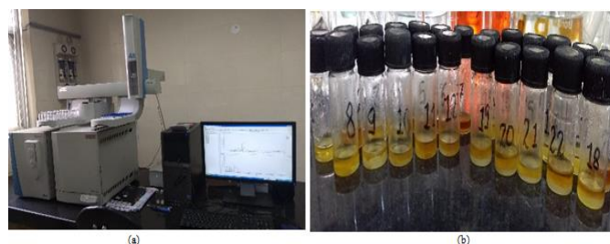
Fig 3: a) GC-MS (Gas Chromatography-Mass Spectrometry) assembly, b) Lemongrass oil
