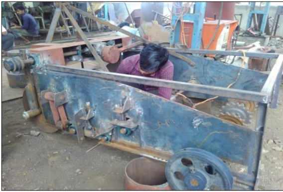
Plate 1: Fabrication of tractor drawn ginger harvester cum elevator
