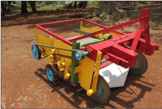
Plate 2: Pictorial view of developed tractor drawn ginger harvester cum elevator
