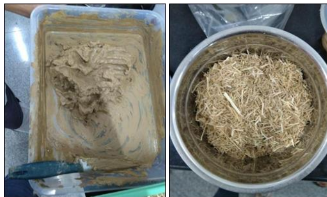
Fig 1: Clay and straw used for the preparation of clay coated carton boxes
