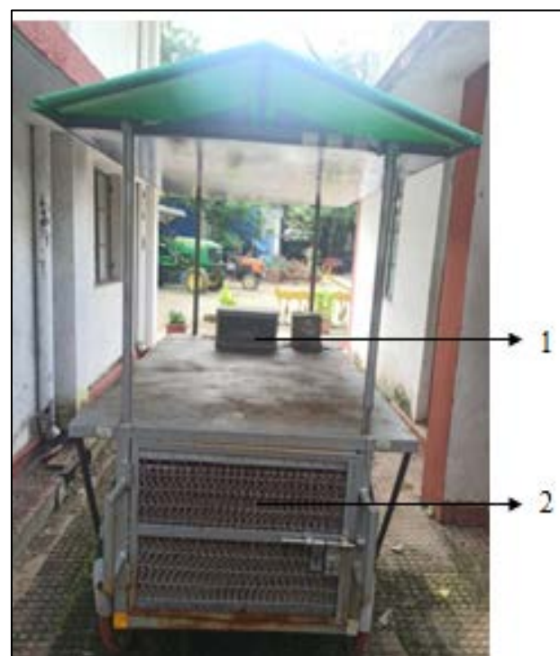
Fig 3: Front view of developed SPV assisted vegetable vending cart 1-Suction fan 2-Loading door
