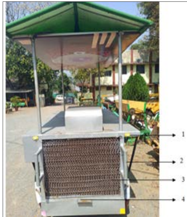
Fig 2: Rear view developed SPV assisted vegetable vending cart 1-LED bulb 2-Handle 3-Cellulose cooling pad 4- Water inlet port
