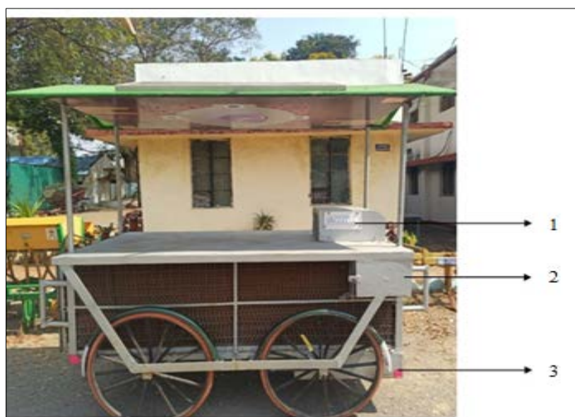
Fig 1: Side view of developed SPV operated vegetable vending cart 1-control switch 2- Battery storage box 3-Water reservoir
