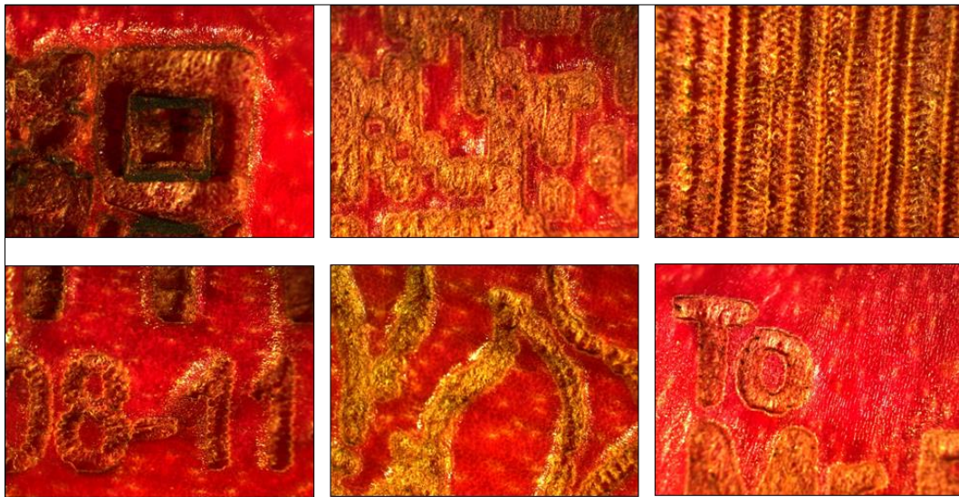
Fig 7: Different types of codes engraved on dragon fruit with laser were magnified under stereo microscope
