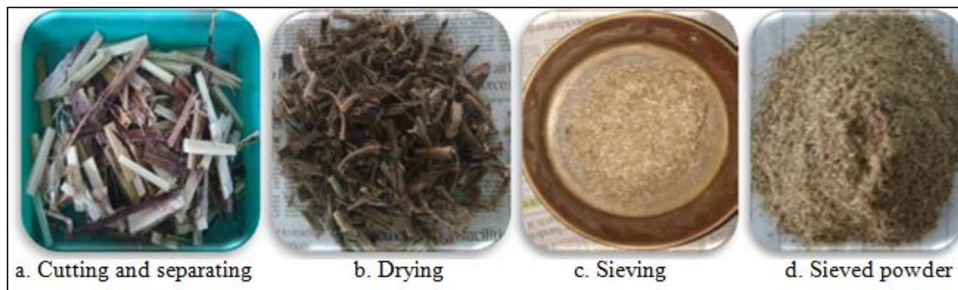
Fig 1: Extraction of fibres from banana sheath
