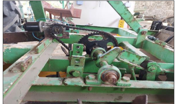
Fig 3: Power transmission with DC motor
