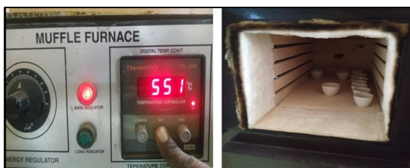
Fig 6: Estimation of Ash content of resin samples in Muffle furnace
