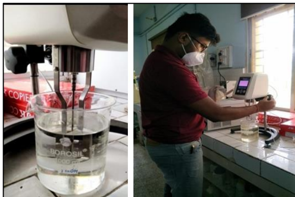
Fig 5: Estimation of Viscosity of resin Samples by using Brookfield DV-E Viscometer
