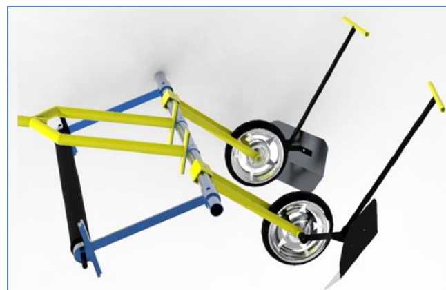
Fig 6: 3-D Solid projection of developed animal drawn plastic mulch laying machine
