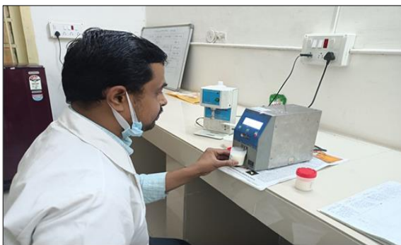
Plate 2: Estimation of milk composition using KSHEERAA-270A automatic milk analyzer
