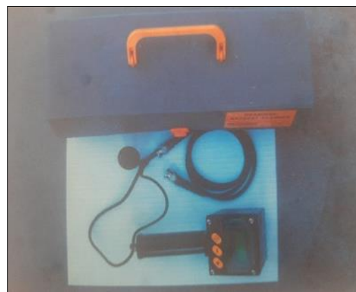
Plate 1: Dramniski back fat scanner for measuring BFT on Live animals
