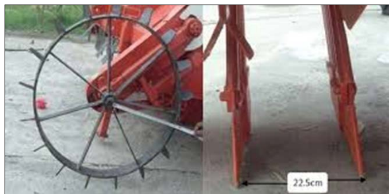
Fig 2: Radius of drive wheel and distance between two furrow openers
