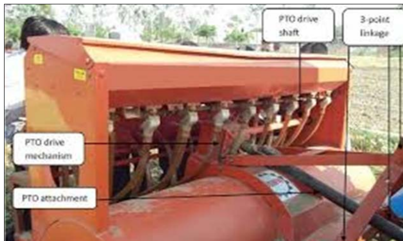
Fig 3: Hitching of the machine through three-point linkage
