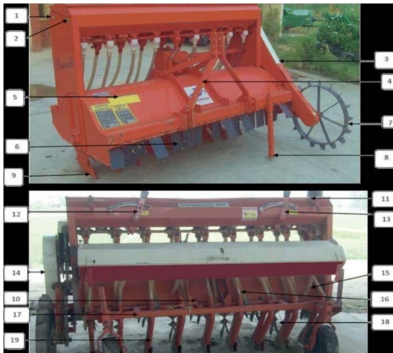
Fig 1: Major Components of turbo happy seeder
