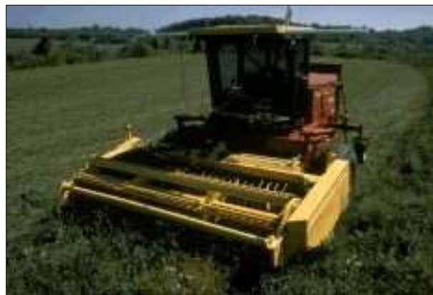
Fig 2: The Demeter automated harvester (Ollis and Stentz 1997) [13]
