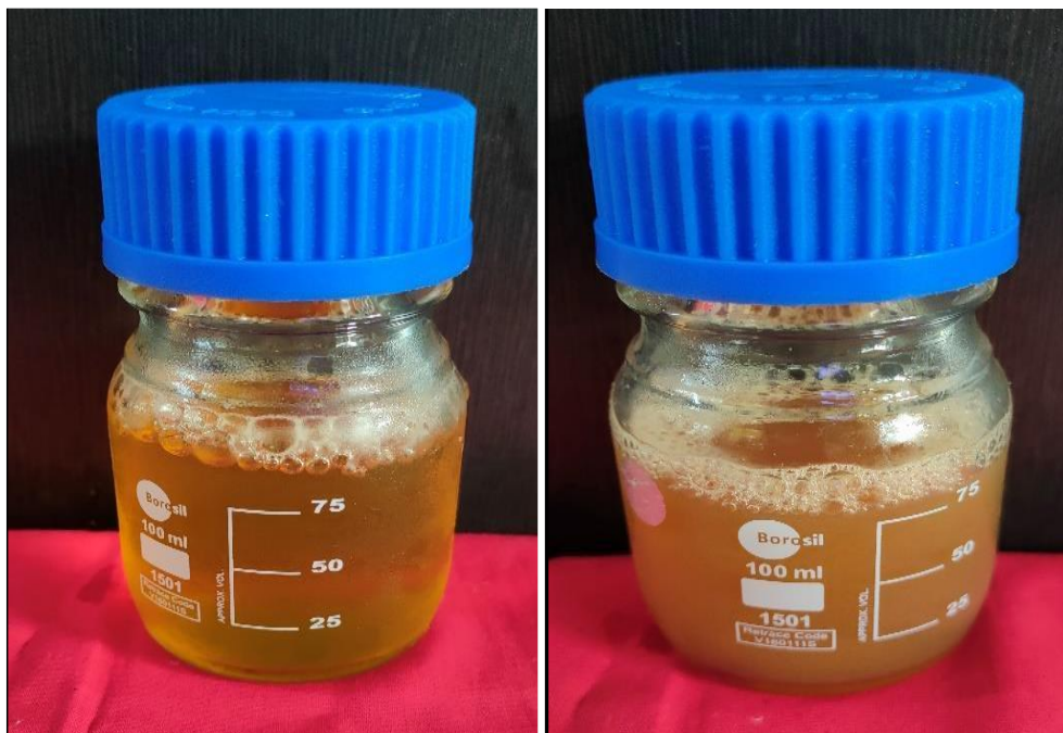
Fig 1: A) Colour change of A. vasica -zinc acetate solution due to zinc nanoparticle formation
