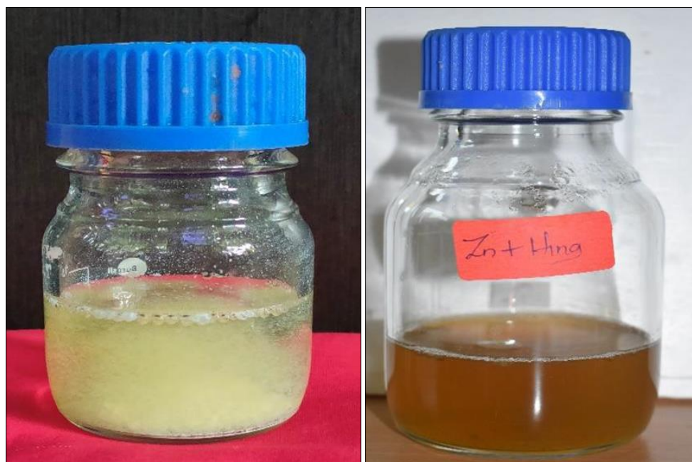
Fig 1: B). Colour change of Asafoetida -zinc acetate solution due to zinc nanoparticle formation
