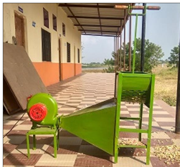
Fig 3: Modified manually operated groundnut decorticator
