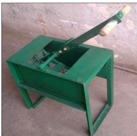
Fig 2: Existing manually operated groundnut decorticator
