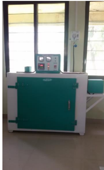
Drying chamber of dryer
