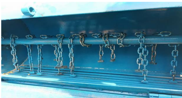
Fig 1(a): Pictorial view of the inside of the shelling drum of maize sheller
