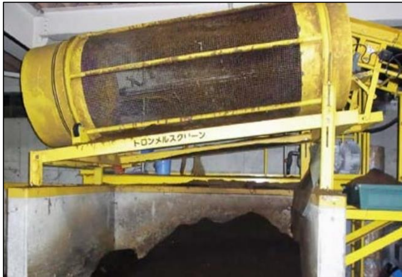
Fig 9: Trommel to remove contaminants
