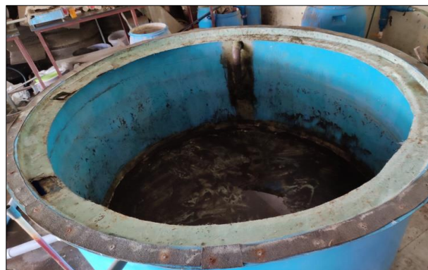
Fig 1: Single stage non-baffled anaerobic digester
