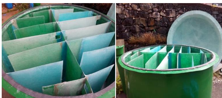
Fig 2a & 2b: Two stage restricted flow anaerobic baffled biogas digester
