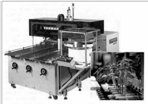
Fig 1: Fully automatic grafting (Suzuki et al. , 1998) [74] .
