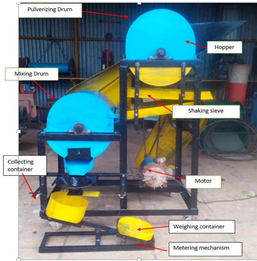
Fig 1: Developed media mixture machine for horticultural crop nursery.
