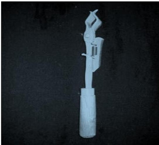
**Fig 2:** Hand tools for de-trashing of sugarcane developed by IISR
