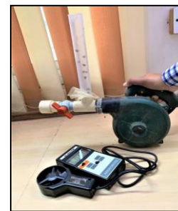
Fig 3: Measurement of terminal velocity by air column method
