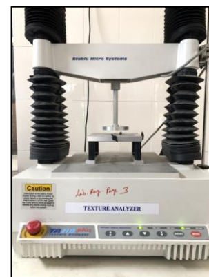
Fig 4: Determination of seed rupturing force by texture analyzer
