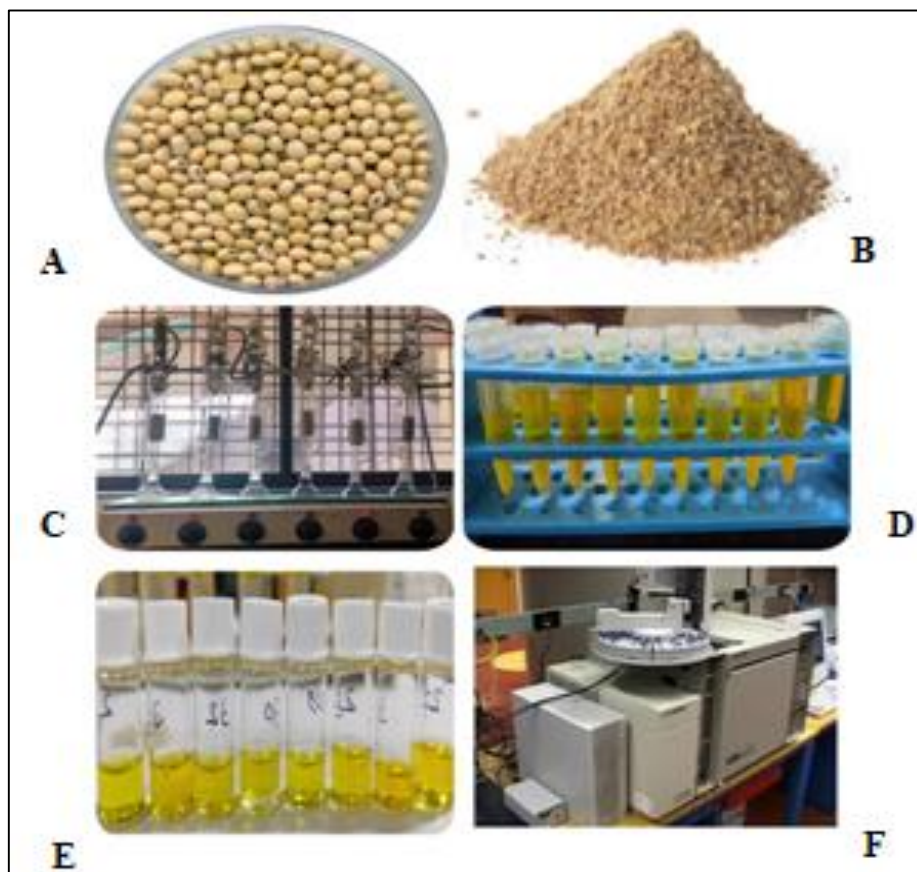
Fig 1: Determination of Total Oil Content by Soxhlet method and Preparation of FAME samples from the soybean matrices A) Soyabean seeds B) Soyabean seed powder C) Soxhlet apparatus D) Oil extracted by Soxhlet method E) Derivatization of oil for GCMS F) GC-MS used for fatty acid Profiling
