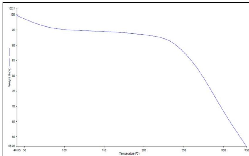
**Fig 2:** Thermal gravimetric analysis (TGA) curves of layer chicken feather fibre (barbs)
