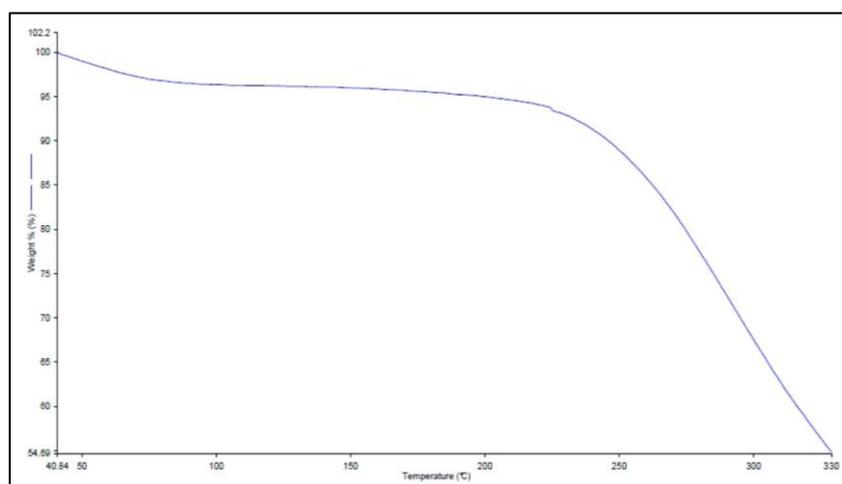
**Fig 1:** Thermal gravimetric analysis (TGA) curves of broiler chicken feather fibre (barbs)
