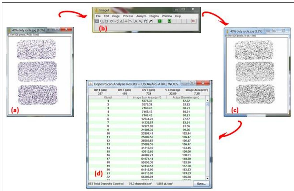
Fig 4: (a) Original scanned color image (b) DepositScan toolbar (c) converted 8-bit gray image (d) results window
