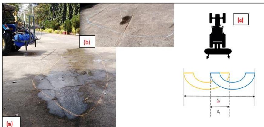
**Fig 2:** (a) marking of wetted perimeter for left spray gun (b) marked wetted perimeters for both the spray guns (c) a typical representation of swath width and overlap.
