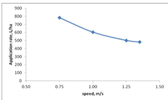
Fig 7: Graph showing relationship between speed and application rate of developed sprayer
