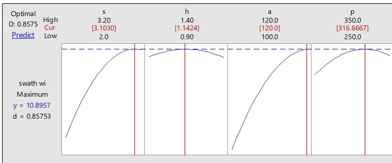
Fig 5: Optimization plot showing optimum operational parameters for effective swath width.
