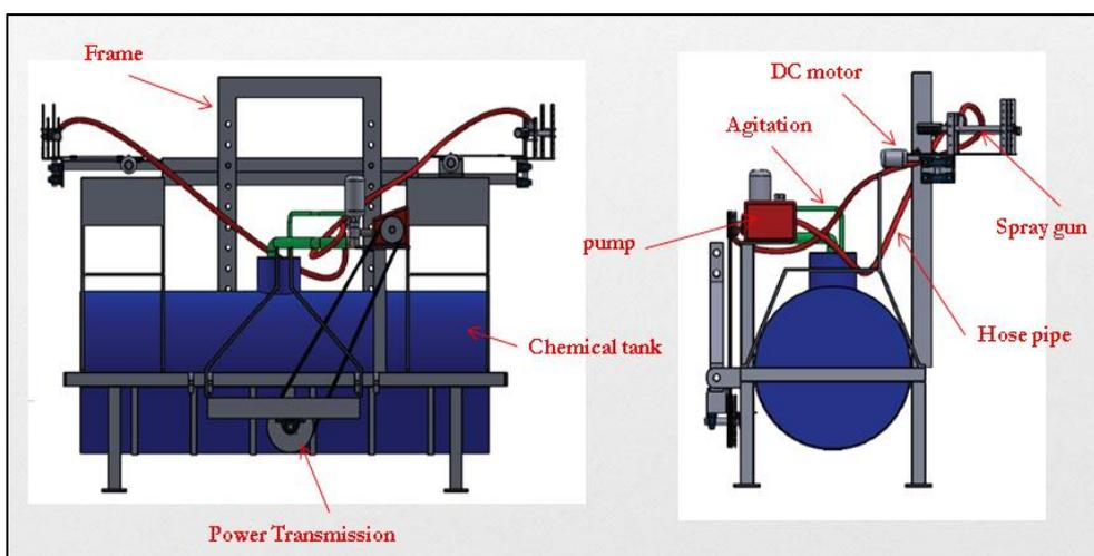
**Fig 1:** Schematic diagram of developed swinging lance sprayer
