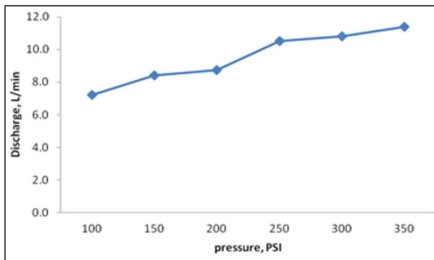
Fig 6: Graph showing pressure and discharge rate relation of spray gun
