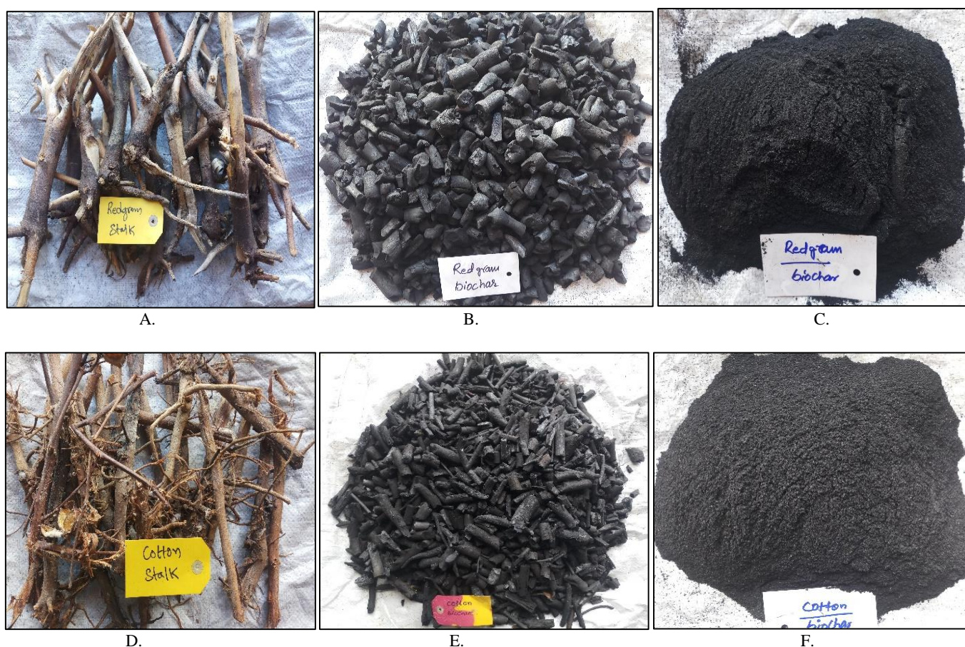
Fig 2: Biochar produced using Drum kiln: (A) Seasoned pigeonpea stalk, (B) Pigeonpea stalk biochar (whole), (C) Pigeonpea stalk biochar (pulverised), (D) Seasoned cotton stalk, (E) Cotton stalk biochar (whole), (F) Cotton stalk biochar (pulverised).
