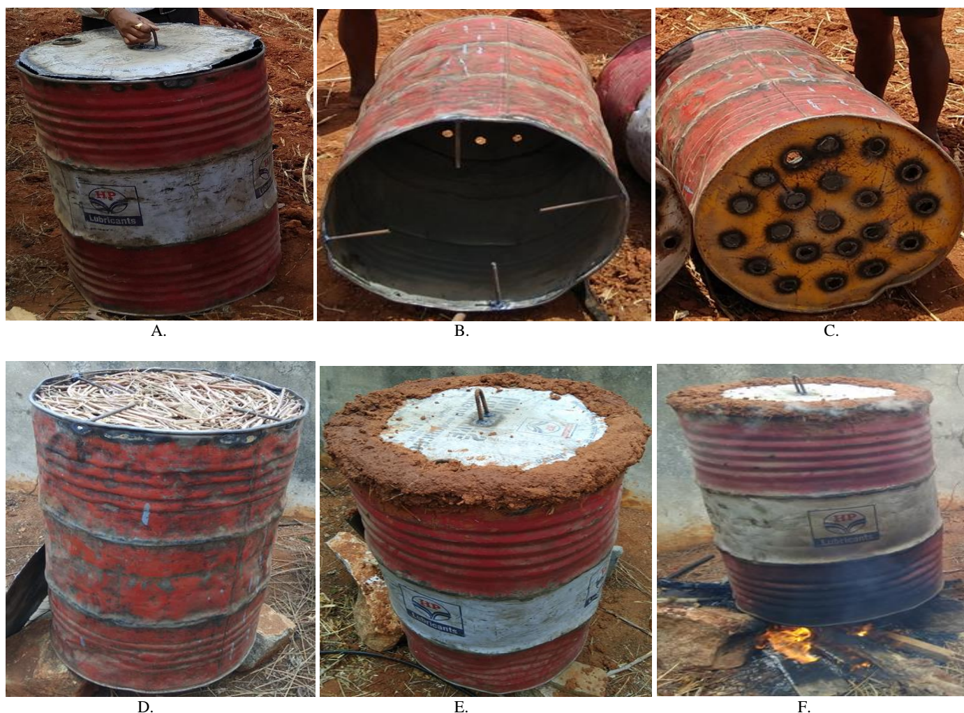
Fig 1: Field operational process of biochar production under drum kiln: (A) General view of biochar drum Kiln, (B) Welded iron sticks at top vent, (C) Bottom view of drum with holes, (D) Drum loaded with feedstock, (E) Drum ready for pyrolysis, (F) Drum kiln under combustion process.
