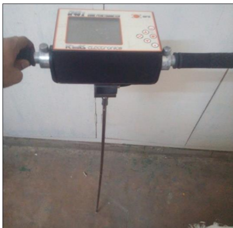
Fig 2: A view of Cone penetrometer
