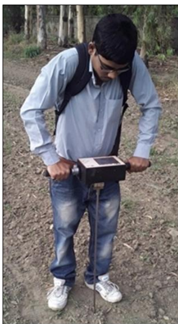
Fig 1: Soil hardness being measured using a digital cone penetrometer
