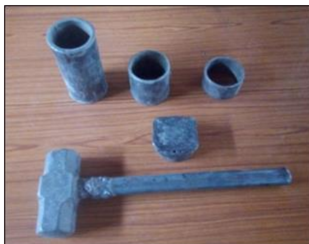
Fig 3: Core samplers along with the hammer
