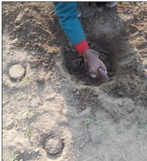
Fig 4: Core samplers excavated out of the soil
