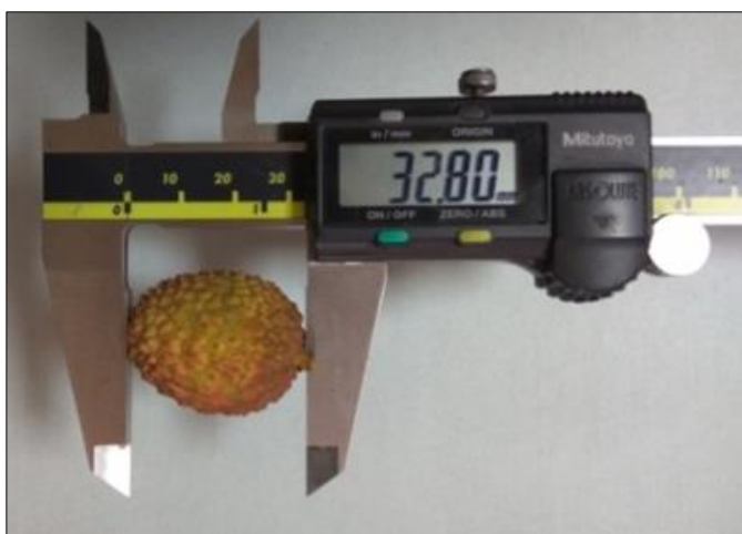
Fig 2: Measuring with vernier calipers
