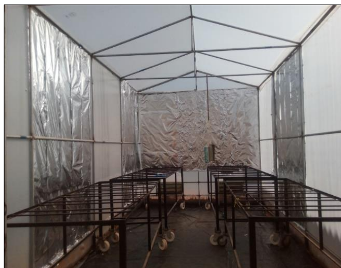
Fig 2: Modified Solar greenhouse dryer using alternate strips of aluminium foil on eastern & western walls, aluminium foil on southern wall and black mulch sheet on the floor
