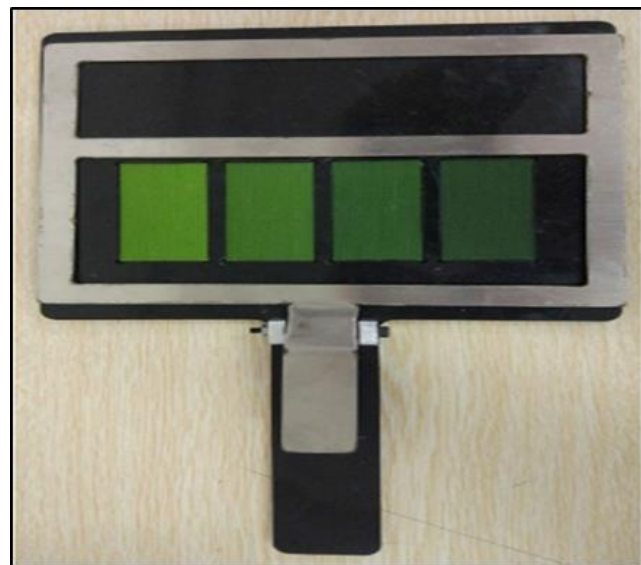
Fig 4: The 4-panel leaf gripper with LCC
