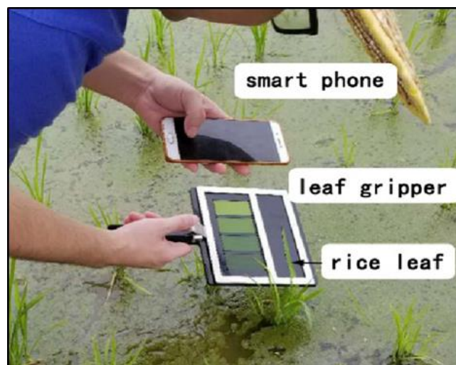
Fig 5: Image taking on the LCC and a leaf in a rice field (Tao et al. , 2020)
