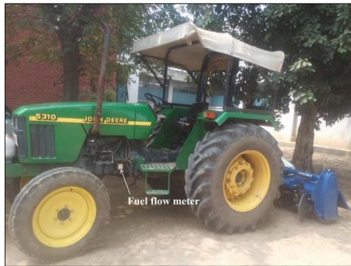
Fig 6: A view of tractor equipped with the fuel meter
