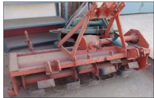
Fig 4: A stationary view of the rotavator with L type blades
