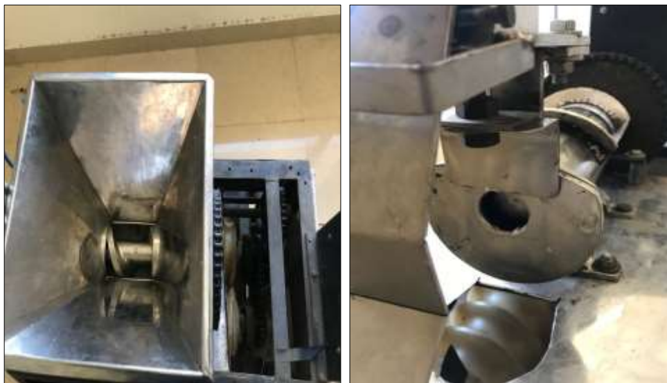
Fig 2: Screw with Hopper (left) and Exit Section (right)
