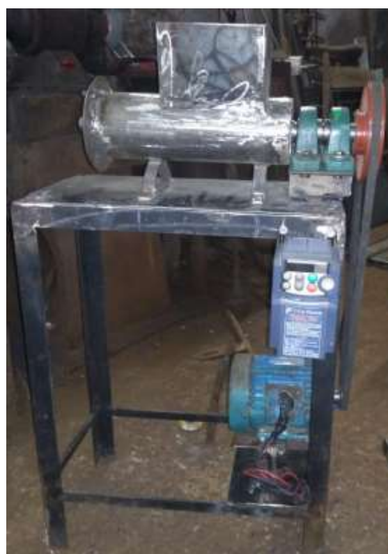
Fig 3: Modified screw mixer (Model 1)
