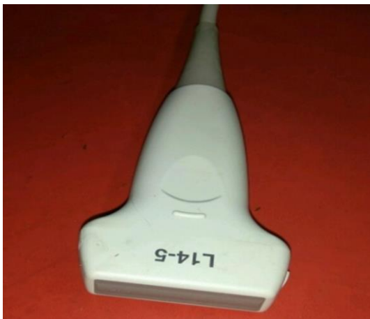
Fig 2: Linear Array Probe (5-14MHz)
