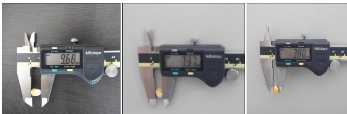
Fig 4: Measurement of length, width and thickness of maize seed
