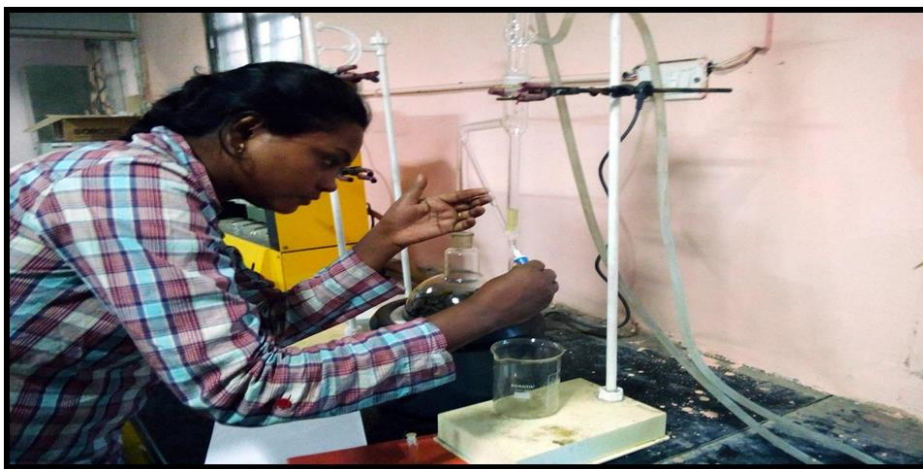
Plate 1: Ocimum basilicum Oil Extraction Process
