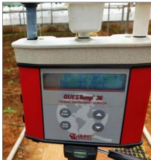
Fig 2: Display screen of heat stress monitor
