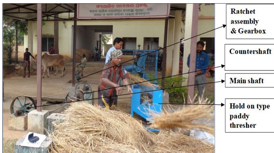
Fig 2: Operation of paddy thresher in bullock operated rotary gear system in CAET campus
